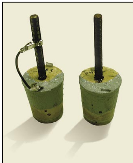
Note rust bubbling out at the base of the rebar on the sample that is not connected to the coating for galvanic protection. These samples were in a humidity chamber for six months.
