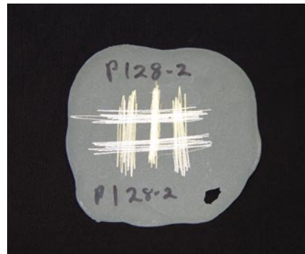
Since GalvaCorr is 90% metal, scratching the surface of the coating will reveal a metallic sheen.
