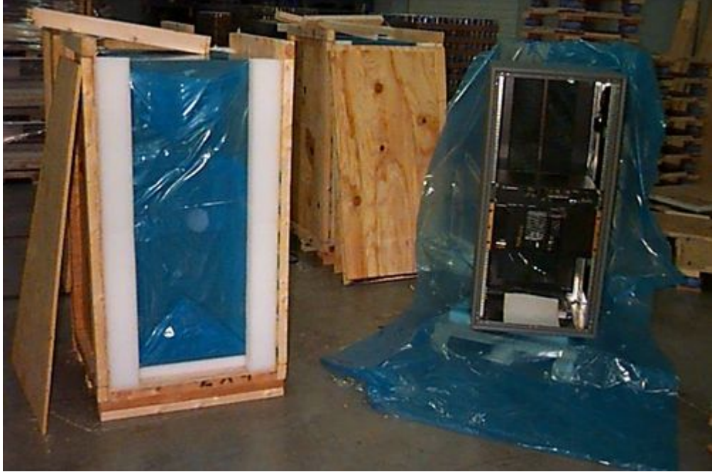
Figure 3. Final Assembly using VCI Technology Company A
