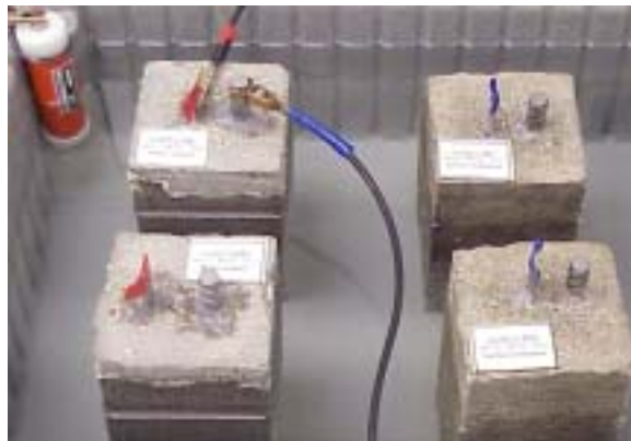
Figure 1. This photo shows four of the concrete samples partially immersed in a 3.5% NaCl solution.
