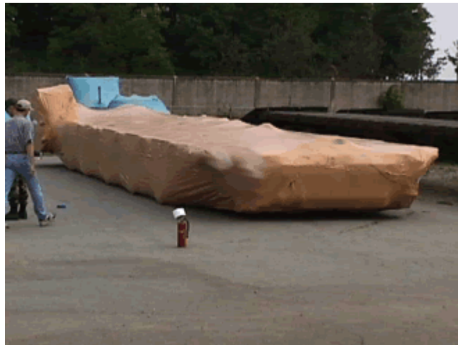
Figure 1. 60K Air cargo loader covered with VCI High UV, Flame Retardant Shrink film.
